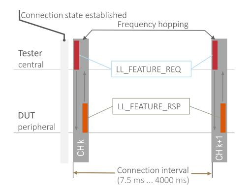
Allows testing of all data channels in frequency hopping sequence with the option to tests only data channels
