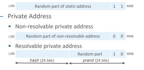
Only public address and static address can be used as identity address
